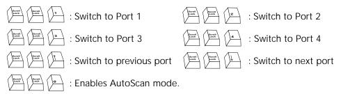
In AutoScan mode, the OmniCube<sup>™</sup> remains on one port for 10 seconds before switching to the next. There is no mouse or keyboard control in this mode. This is necessary to prevent errors. Otherwise, if the user is moving the mouse or using the keyboard when the OmniCube<sup>™</sup> switches to the next port, data flow is interrupted and will cause erratic mouse movement and/or the wrong characters to show up when using the keyboard.
